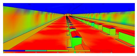
Try to eliminate shadows between nests by using sufficient rows of lights and lights per row.
