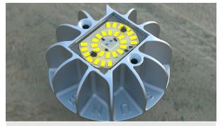
A 10W LED luminaire with aluminium heat sink and aluminium PC board for maximum heat dispersion resulting in a longer product lifespan.
