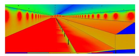
*Light is brighter against the walls. No shadow at step. Linear uniformity is excellent. Note how lux diminishes closer to the nest.*
