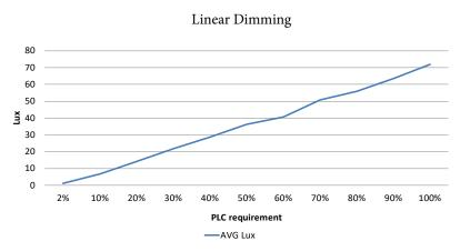
A linear dimming curve makes for simple programming of your PLC: 0V = Off, 5V = 50% and 10V = 100% output.
