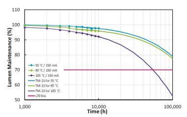
Note how the 105°C LED drops below the 70% before the 55/85°C LED in this example.
