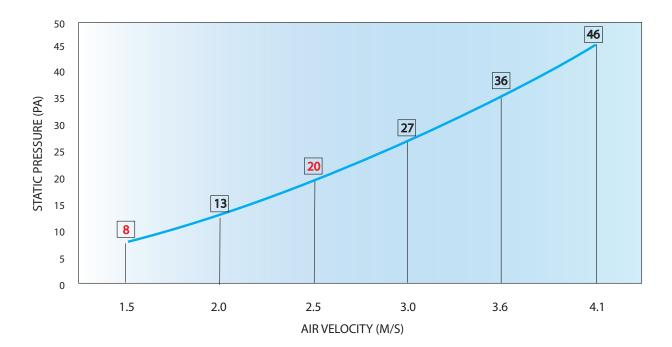
Vertical blade type light trap resistance to airflow in Pa and m/s Light reduction factor - 1,900,000 : 1
