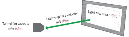
Light trap area  $m^2(ft^2)$  = Tunnel fan capacity  $m^3/s$  (cfm) ÷ Light trap face velocity m/s (f/m)
