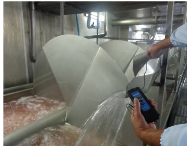
Factors in chilling that affect moisture absorption include water temperature, flow, and agitation
