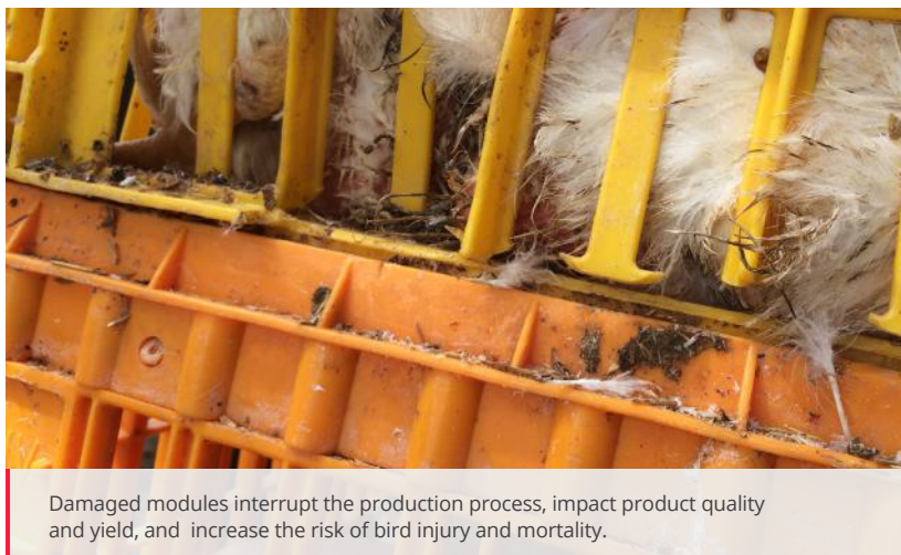
Transport modules should have no cracks, breaks, or damage and should be clean prior to loading.
