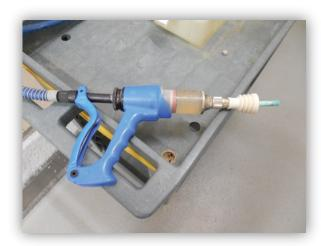
**Figure 1:** A hand held device where the dosage can be changed with a dial. The end of this device is placed at an insertion point on the hatcher cabinet to then place formaldehyde into the cabinet.
